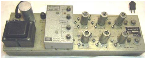
Figure 5. Vacuum Tube Technology: the Jerrold 12-Channel SDA-4 Super Distribution Amplifier
