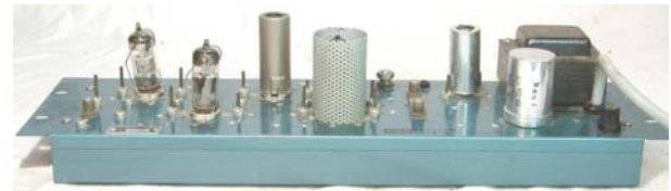
Figure 6. Vacuum Tube Technology: the Jerrold HPM-12 Channel 12 Amplifier
